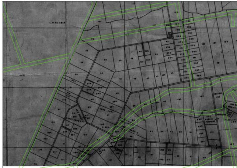
Figure 2: Buffer zone of road-centre line datasets (in green) superimposed on a parcel boundary dataset.
