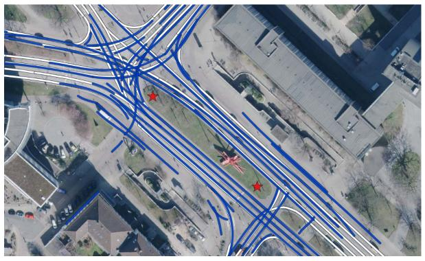
Fig. 10: Comparison of manually labeled (white) and automatic detected (blue) lane axes. Ortho image: (HANNOVER 2017)
