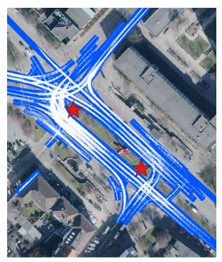
Fig. 1: Data and results of our experiment: trajectories (white), lane segments (blue), scanner positions (red). Ortho image: (HANNOVER 2017)
