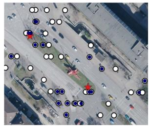
Fig. 7: Geo-referencing, manually measured poles (white circle), automatically detected poles (blue circle) and scanner position (red stars). Ortho image: (HANNOVER 2017)
