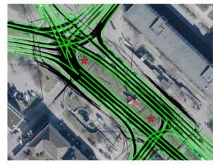
Fig. 3: Trajectories (black) and reference lane markings (green). Ortho image: (HAN-NOVER 2017)
