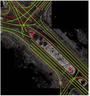
Fig. 6: Reference data lane borders (red lines), middle axis (green lines) and poles (red points)
