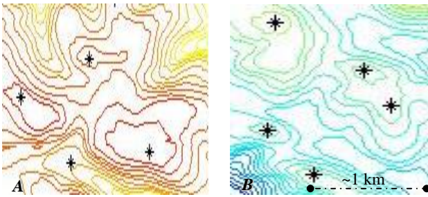
Figure 7. Contour representation showing effective identification and extraction of local geomorphologic surface-derived points
