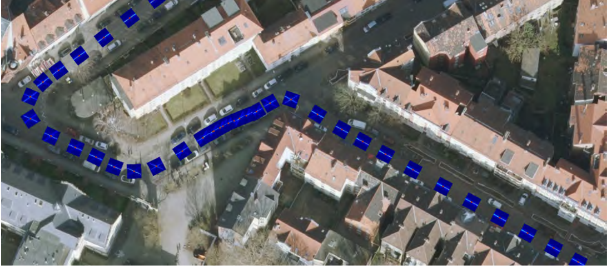
Figure 5.7.: Application of the maximum consensus localization: For a section of the Nordstadt trajectory, the 2D maximum consensus accumulator slices of the optimal heading angle are visualized on top of an orthophoto. Every 20th epoch is illustrated, the size of the 2D xy -grids is 4\text{ m} \times 4\text{ m} , and the red dots indicate the localization solutions.
