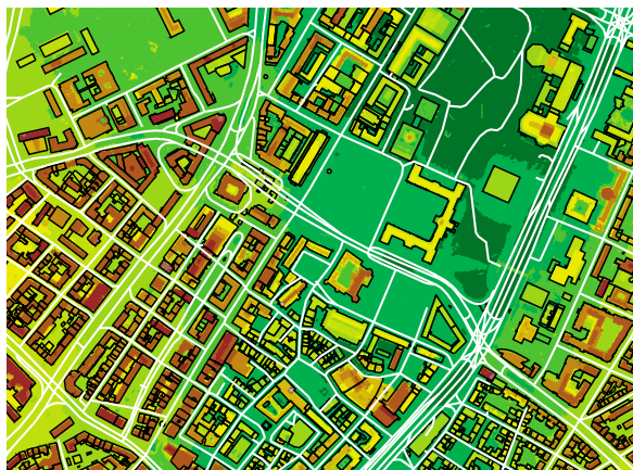
Figure 2: Laser scan (regularized to 1 m rasterwidth, shown color-coded), streets from GDF dataset (white) and building groundplans from cadastral map (black). Image shows part of Stuttgart, Germany.
