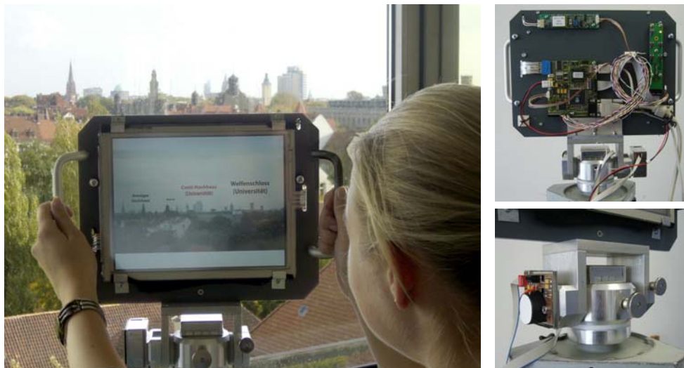
Figure 2: Snapshot of the GeoScope prototype, front side (left), back side (upper right), compact two axes head with angular measurement units (lower right).
