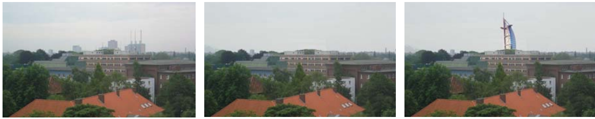
Figure 5: Example for an overlay of a real image and virtual contents. Left: original image, centre: masking, right: real image with overlaid virtual content.
