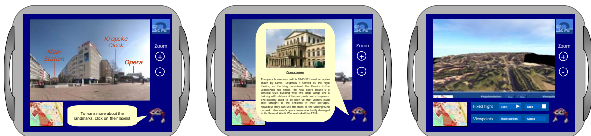
Figure 4: Examples for simple display and interaction techniques: panoramic view with overlaid virtual labels (left), textual description of a landmark appearing after a label has been selected (middle), purely virtual flight controlled by the GeoScope's pan and tilt angle (right).
