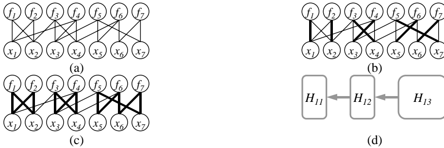
Figure 2: Constraint graph for Eq. (3). (a) Original graph, (b) perfect matching, (c) strongly connected components, (d) collapsed graph H .
