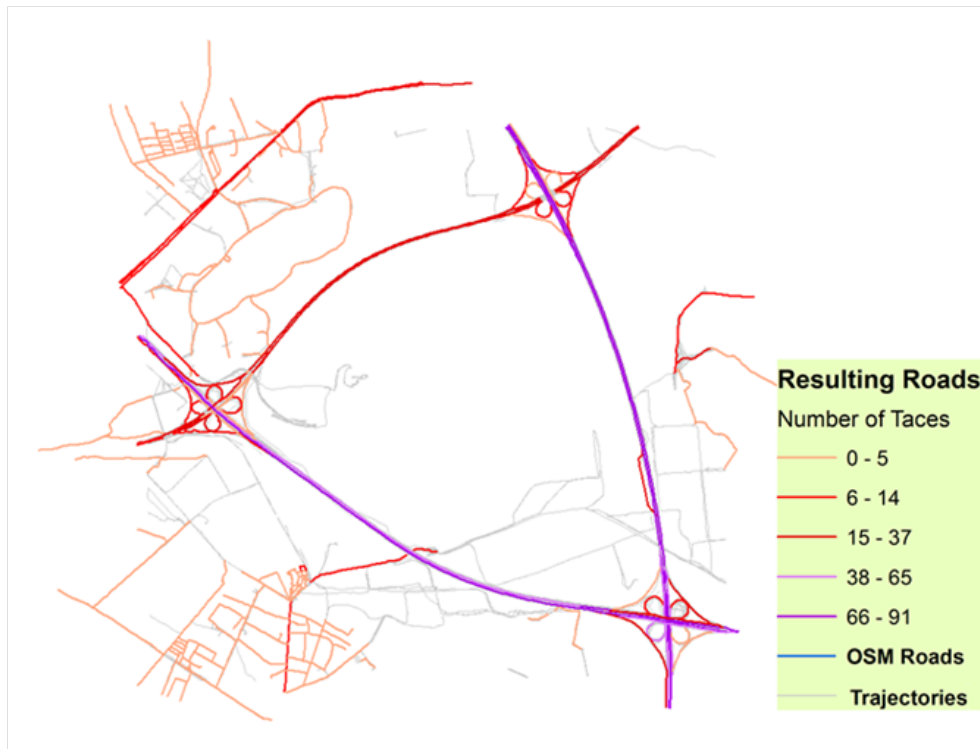
Figure 7.6: Resulting roads constructed from GPS-trajectories.
