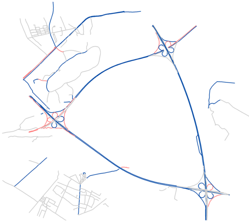
Figure 7.10: Experimental results of estimating the number of lanes. Roads that are given the correct number of lanes are presented in blue and wrongly estimated roads are in red. Roads that have less than 3 roads are presented in grey.
