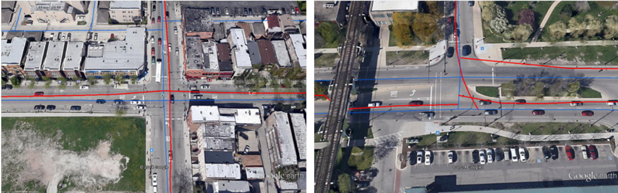
Figure 7.13: Two examples of the constructed road map. Roads are overlaid on Google Earth image data. Prior map is shown in blue, and red lines are the resulting roads.
