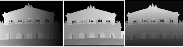
Figure 4: Laserscan of the opera in Hannover represented as x, y and z image
