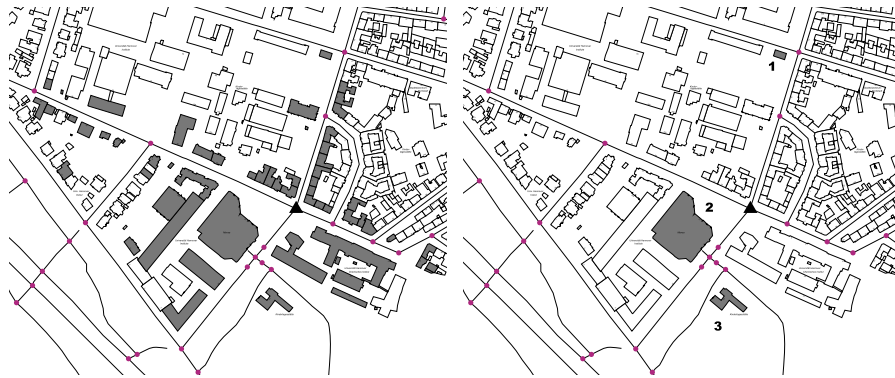
Fig. 2. Decision point (black triangle). Left: selection of all visible buildings. Right: three potential landmarks after processing.
