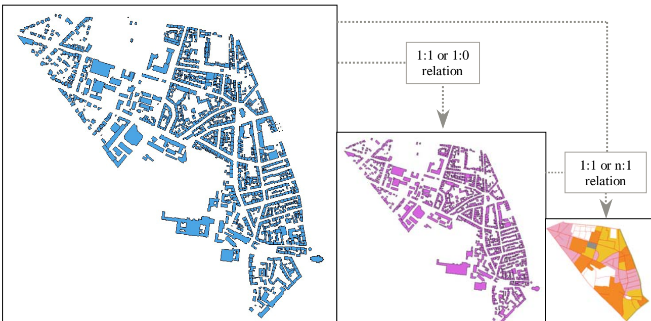
Fig.7: Three stages of the MRDB: a) original buildings, b) generalised (simplified) buildings, c) built-up areas Data from ALK ® (courtesy of Mapping agency of city of Hannover) and ATKIS ® Germany (courtesy of LGN, Hannover)
