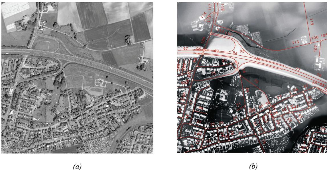
Figure 1. (a) Orthophoto of test area, (b) cartographic map data draped onto digital surface model (DSM)
