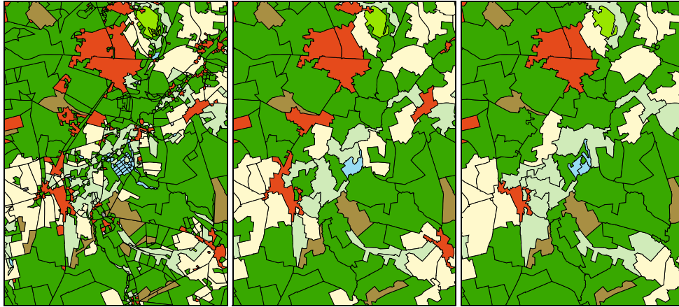
Fig. 3: A sample from the ATKIS DLM 50 (left), a result of the heuristic developed by Haunert (2007b), and a result of a simple iterative merging procedure (right). Both results satisfy the specification for the ATKIS DLM 250.
