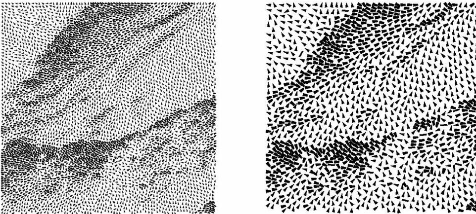
Figure 2: Buffered, normal based textures, applied on the DTM-AV. Left: 2 pixel distance, scaled, size 4x8 pixel. Right: 1 pixel distance, size 8x16 pixel.
