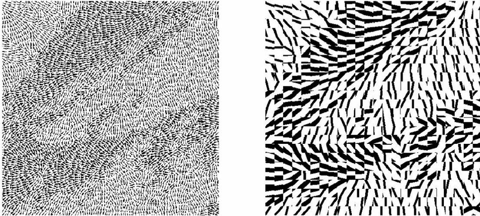
Figure 1: Normal based, pixel-wise texture assignment for the DTM-AV. Left: Triangles, width 5 pixels, scaling factor 10. Right: Rectangles, width 10 pixels, scaling factor 20.
