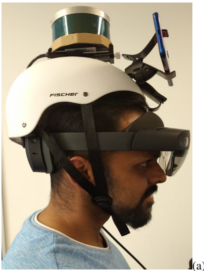
Figure 2: (a): Pedestrian with the social distancing helmet, (b): Different components of the SDH interacting with the system
