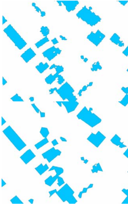
Figure 9 : Example of a larger area: original building outlines (top); adjusted straight lines (bottom).
