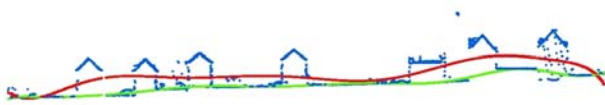
Figure 2: Side view of the selected profile (blue) and the adjusted polynomial after one iteration (red) and five iterations (green).
