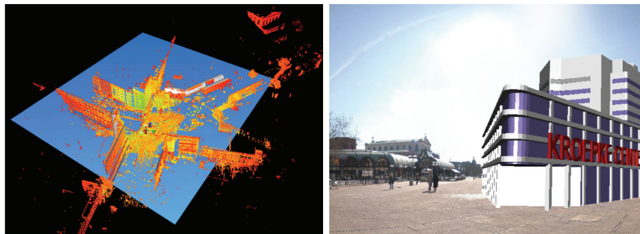
Figure 4: Planning application: depth map for occlusion (left); image overlay (right)
