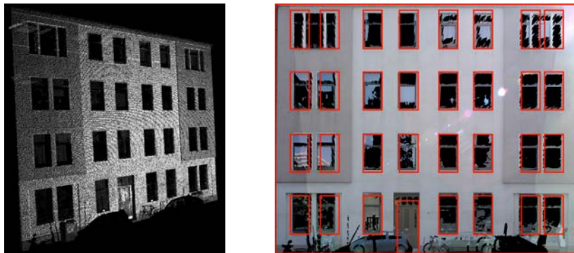
Figure 8: Point cloud of a facade and the reconstruction result visualized in the orthopoto.
