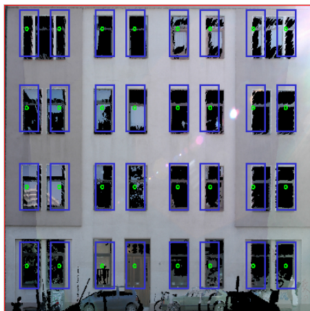
Figure 17: Facade model with a grid of window pairs.
