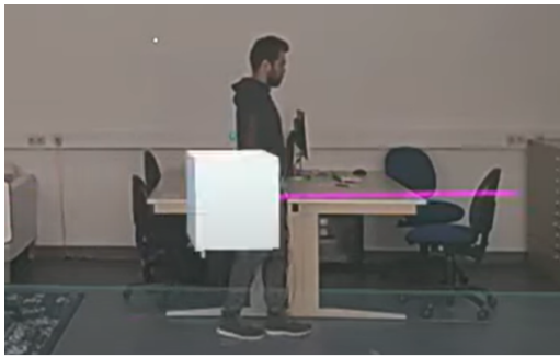
Figure 2: Each detected person in the view of the Hololens user is visualised in Unity with cube and future direction indicator
