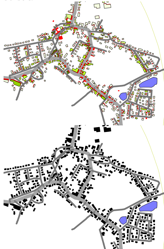
Figure 8: Displacement: Overlay of original objects in conflict (top) and solution after automatic displacement.
