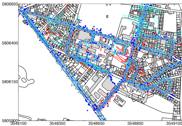
Figure 6: Landmark based positioning for ahead and oncoming vehicles and GNSS based ego position for selected vehicle position (cyan) versus only landmark based positioning (red).
