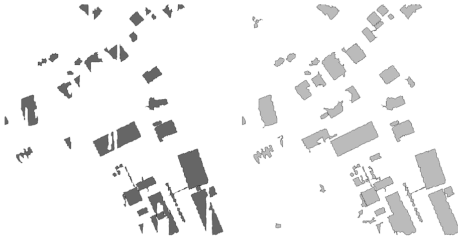
Fig. 5. Result of the classification and segmentation of off-terrain points. Left: polynomial estimation with degree 20 (starting at degree 5). Right: Mixed classification using polynomials between degree 5 and 20.
