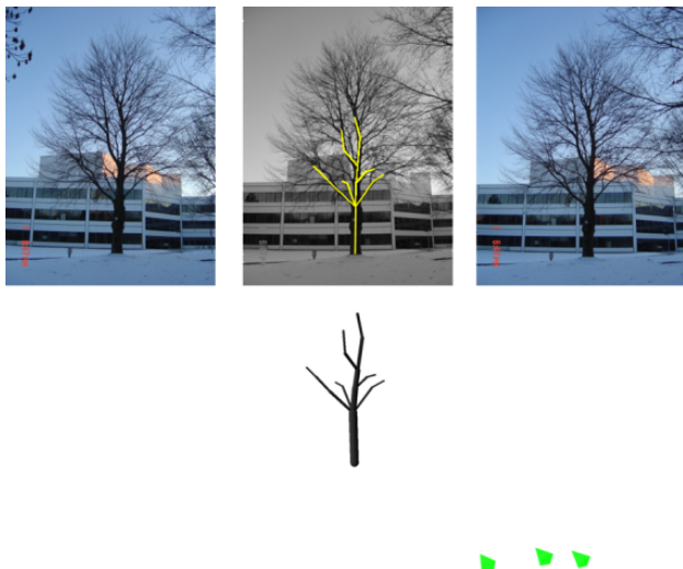
Figure 3: Result for a symposiumal-monochasium tree limited to the trunk and the first several levels of branches – image triplet (top), a snapshot of the search process (top-center), and the result as a VRML model (bottom). The cameras are shown as (green) pyramids.
