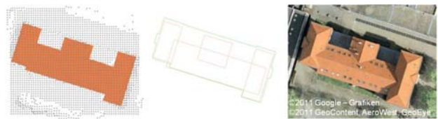
Figure 7. Building parts with lower roofs and smaller extrusions have not been reconstructed: footprint in point cloud (left), comparison with given ground plan (middle), and an aerial image as reference (right)
