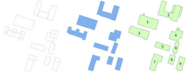
Figure 6. Footprint reconstruction of a scene with multiple buildings: the extracted primitives (left), reconstructed footprints (middle), and the ground truth data (right) from cadastral map as reference
