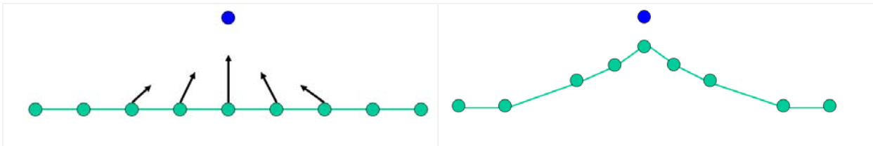
Figure 2: One-dimensional situation: stimulus (dark color) triggers a change of weights (position) of the neuron chain (in light color) and their neighbors; result of adaptation (right).
