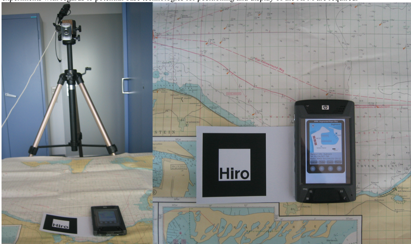
Figure 5: “On paper” concept evaluation prototype using a PDA and marker-based positioning
