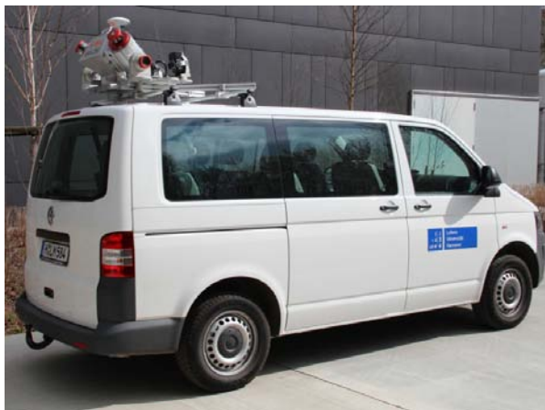
Abb. 2: Riegl VMX-250 Mobile-Mapping-System
