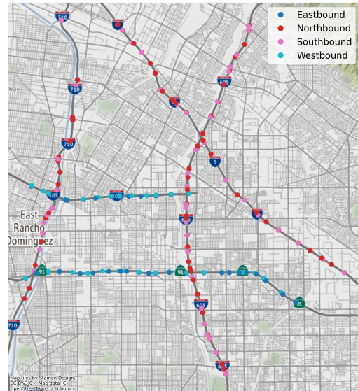
Figure 4: The location of the selected sensors in the PEMS dataset. The colors indicate the direction of the road on which the sensors are placed.
